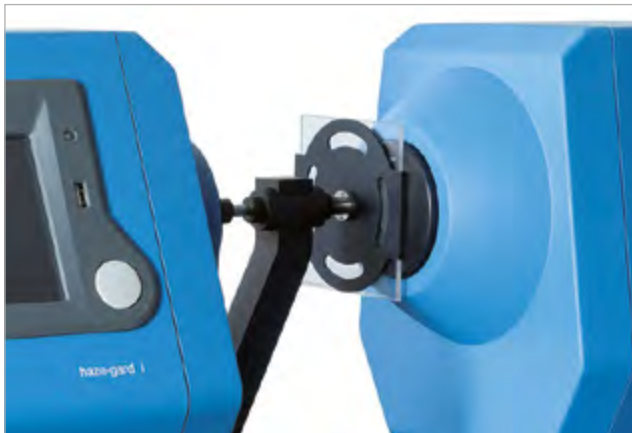
The measurement of haze is used to determine abrasion resistance of transparent materials. The haze-gard i Abrasion Holder facilitates positioning of the abraded area in the measurement beam.
