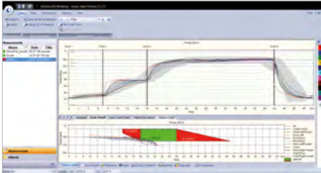
temp-gard collects temperature data in production oven.
