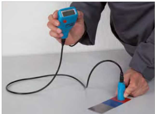
byko-test with extension cable
